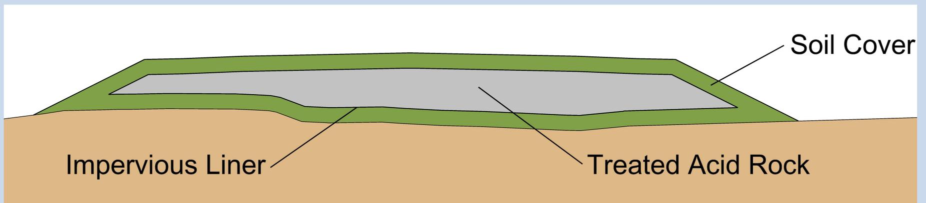
Typical section of treated acid rock with impervious liner and encapsulated.
